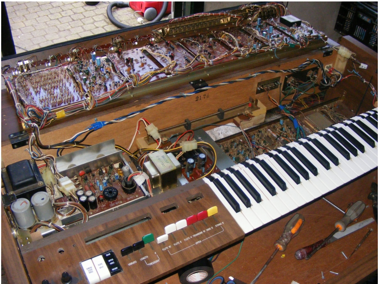
Fig. 3: This picture shows how several parts where moved into the upper part of the housing. For instance: the power supply(left), reverb spring (middle), power switch and outputs (upper right).
