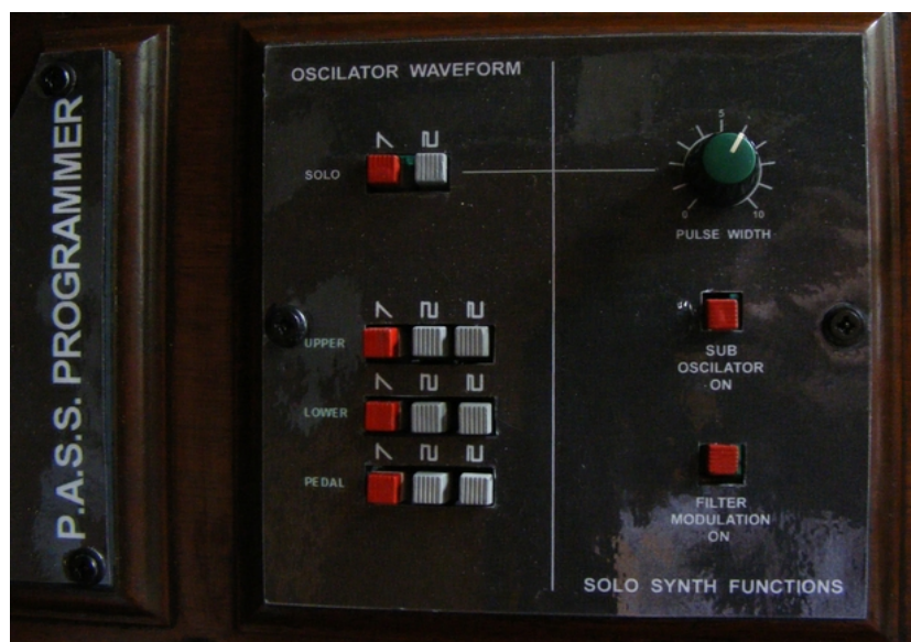
Fig. 8: The new left main panel with the waveform selectors and additional solo synth controls on my own SGX V2. Point 5 in paragraph 13 however describes a much easier fix.
