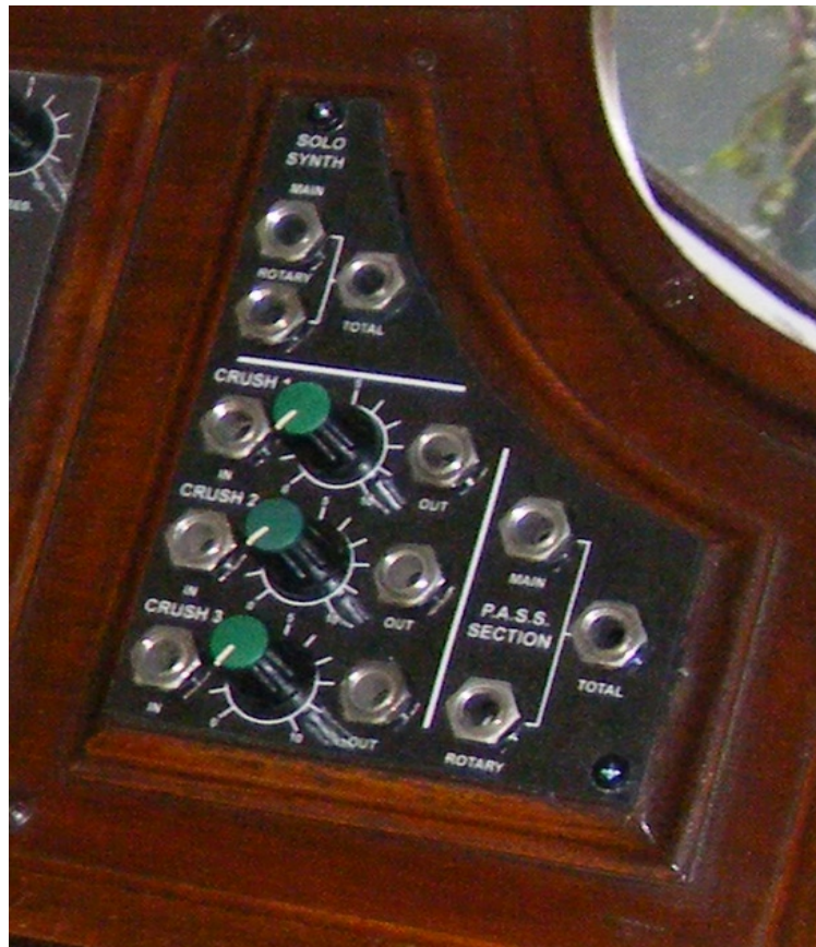
Fig. 11: The far right panel on the programmer box contains the individual outputs and the in and outs plus control pots of the 3 audio crushers.
