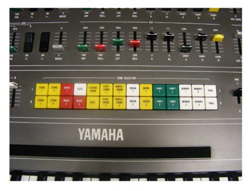
Up to the next slider. This one determines the mix between the upper channel (channel 1) and the lower channel (channel 2). If the fared is set fully to the upper channel only that is heard. If the slider is pulled fully down only channel 2 sounds. Any setting in between leads to a mix of both sounds. The middle setting means both sounds are amplified equally strong.
